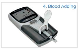
Press the sampler thread (with sample) onto the strip
